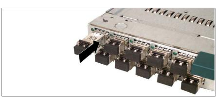
Figure 55: Inserting an SFP module
